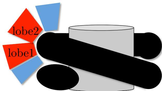
FIGURE 4 Schematic drawing of the remodeler engagement for the Snf2-construct, following Fig. 3 *a* from (39) and Fig. 2 from (40). The color scheme is as follows: light gray, histone octamer; black, nucleosomal DNA; lobe 1, lobe 2: ATPase units. The remaining trapezoids sketch accessory remodeler domains. To see this figure in color, go online.
